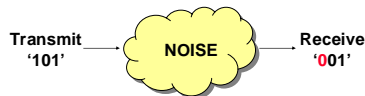
Figure 1 – A simple model of the effects noise can introduce into a transmitted signal.
